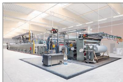
Picture 3: A typical integrated Monforts coating line is automated from the inlet feed to the winder
