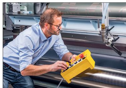
Picture 1: Adjustments can be made simply and easily with the new hand-held remote controller which has recently been introduced for the Montex®Coat unit
